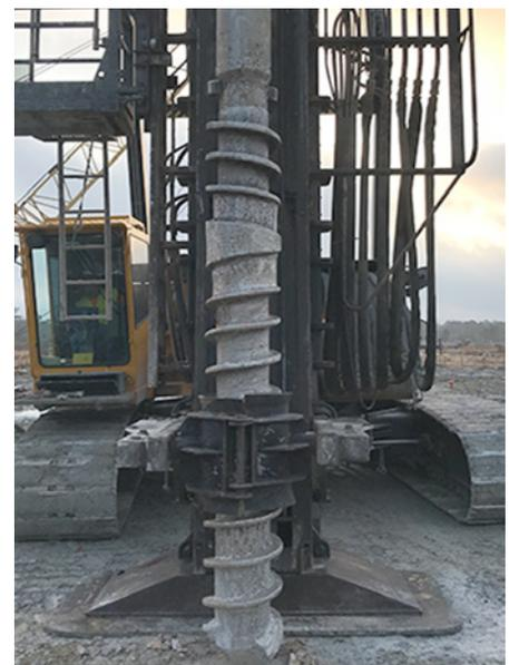
Morris-Shea DeWaal Pile drilled displacement tool
